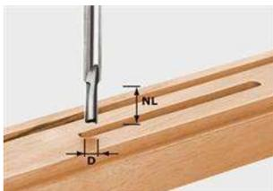
**Festool Nutfräser D3mm/NL6mm/GL45mm/S8mm
