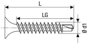
**Spax GIX-D Trockenbauschraube Ø3,5x25 mm
